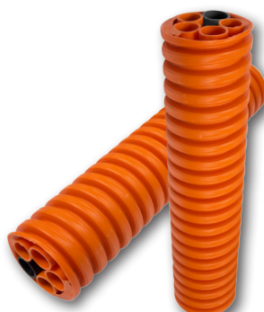
Ø 110 mm with 33mm x 5 sub-duct
